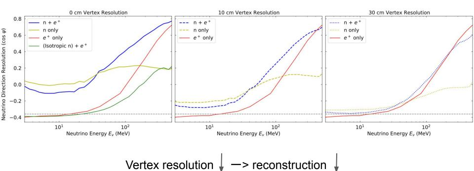
Neutron diffusion in water makes it impossible to reconstruct at the event-by-event level but possible to statistically infer the direction of the neutrinos using multiple events
