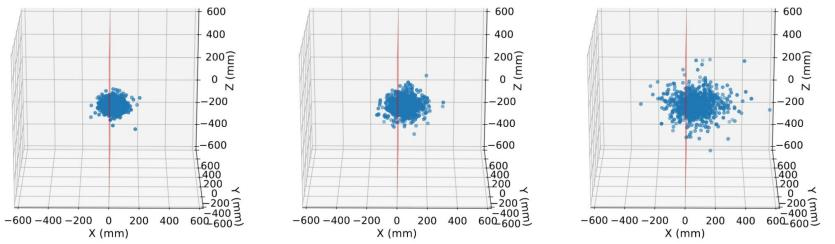
Neutron capture positions in Gd-loaded water 20 MeV (left), 50 MeV (middle) and 80 MeV (right) neutron momenta are emitted along the x-axis
