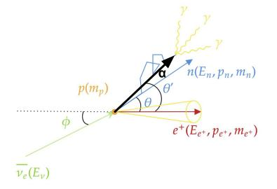
A neutron vector constructed by connecting the original point and the capture position point.
