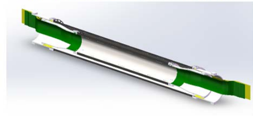
Fig.13 The inner two layers of half bent MAPS cylinder: no contact between layers.
