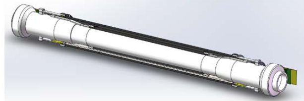
Fig.14 The inner two layers of half bent MAPS cylinder-no contact between layers.
