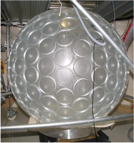
Acrylic vessel of diameter 1.7 m which contains ~ 3.3 tons of liquid argon.
