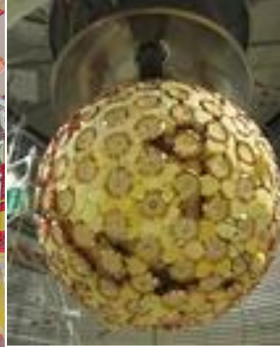
Detector with PMT installed & during backing foam (yellow) installation
