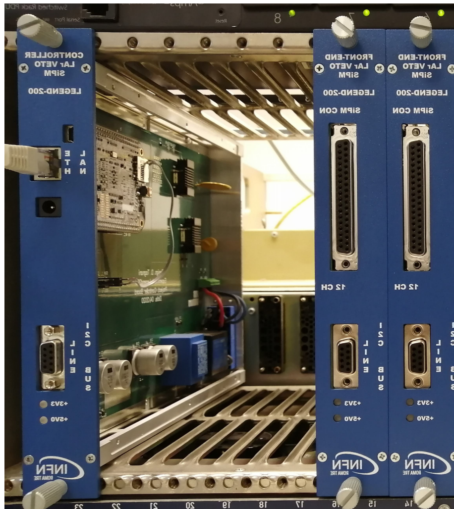
LEGEND-200 FE boards x 2 & controller board
