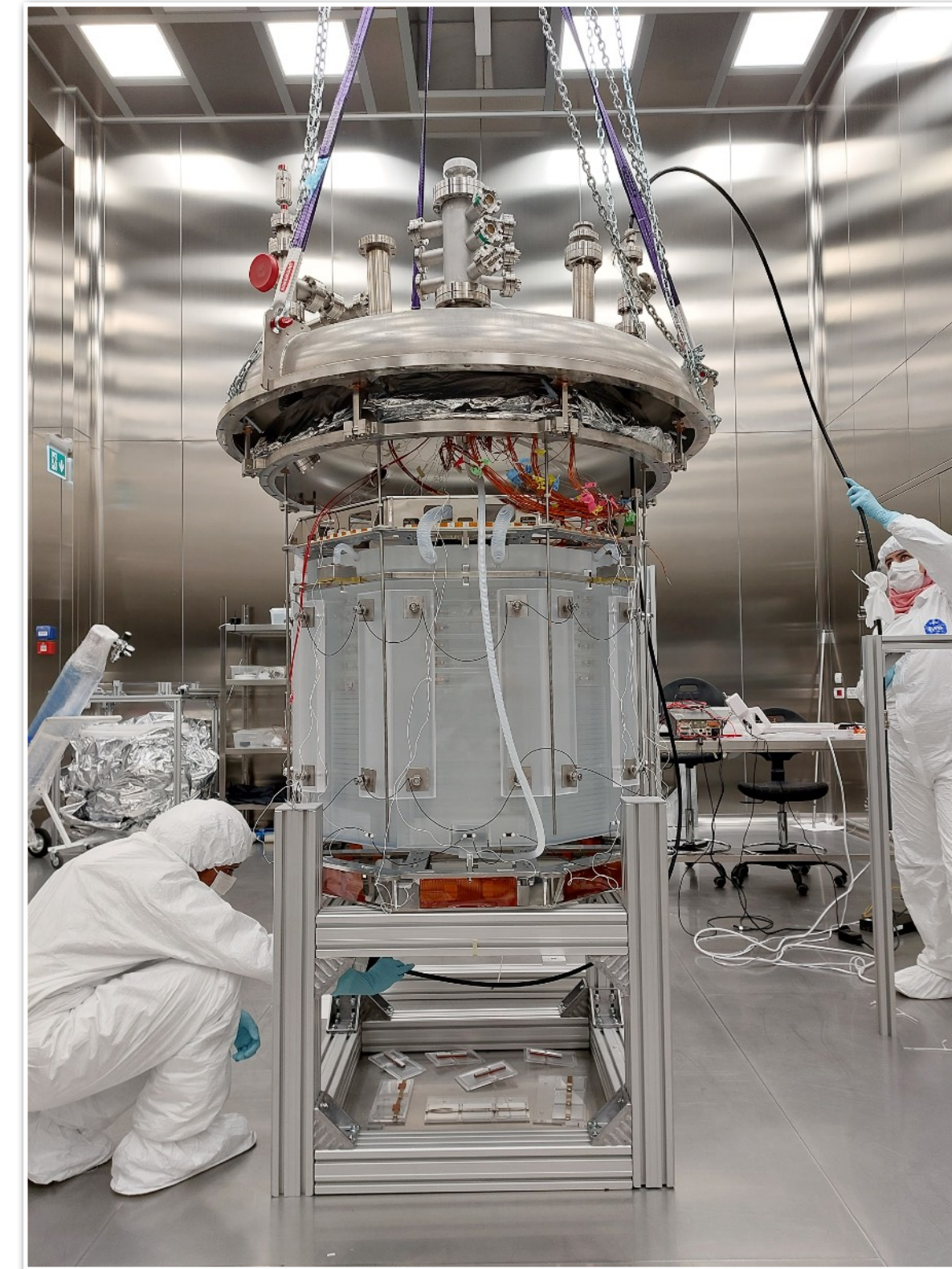
Cryostat dome connection
