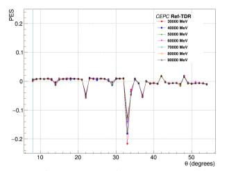
In the center of modules (barrel or endcap), scale value is almost at 0, need calibration for cracks - One point with long error bar (fit problem)
