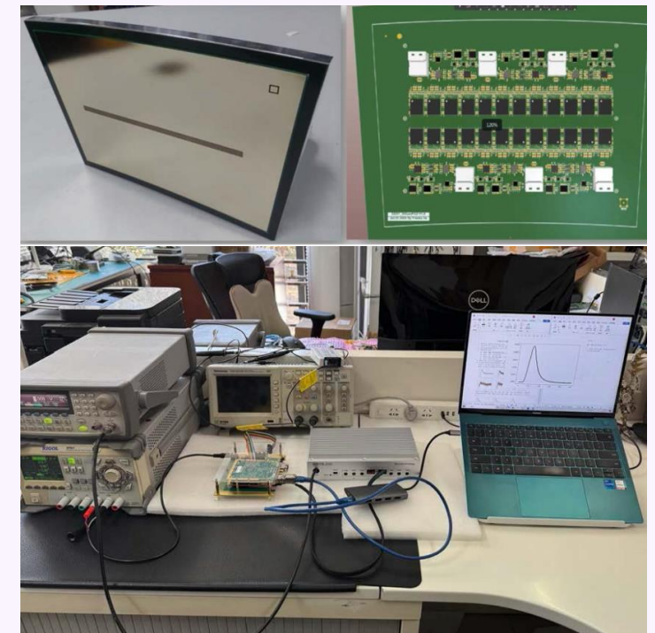
TPC modules assembled for the beam test
