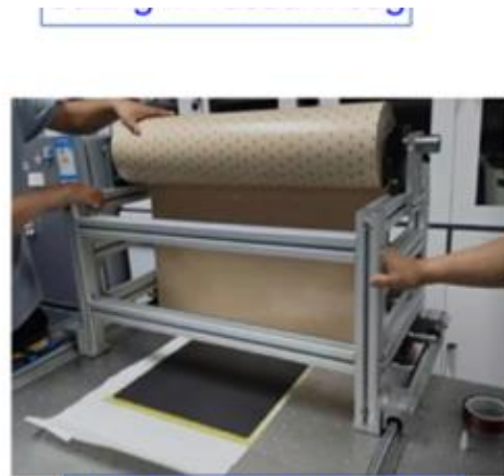
Applying insulation film
