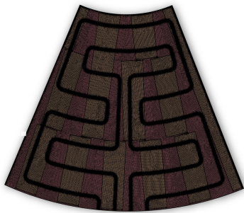
1/8 ITK endcap cooling loops
