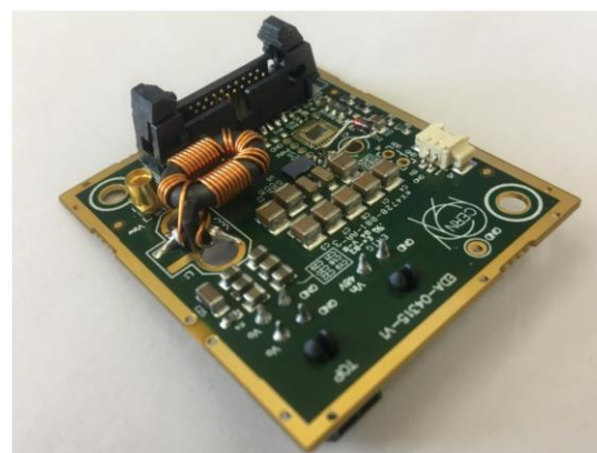
Figure 17: bPOL48V using the FEASTMP inductor.
