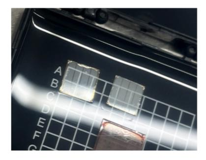
Single-crystal diamond Size: 7.64mm \* 7.58mm Thickness: 222µm
