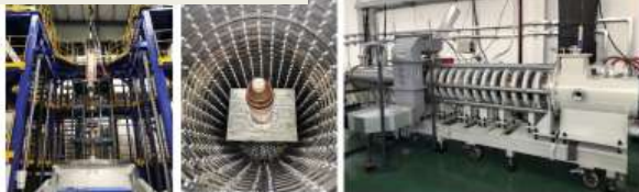
Klystron No. 1 Efficiency 65% (2020)
