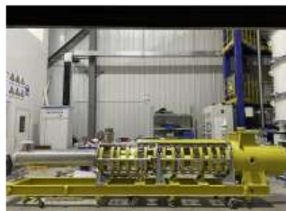
Klystron No. 2 Efficiency 77% (2021)
