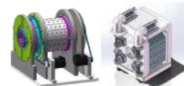
Permanent quadrupole's prototypes for CEPC collider rings
