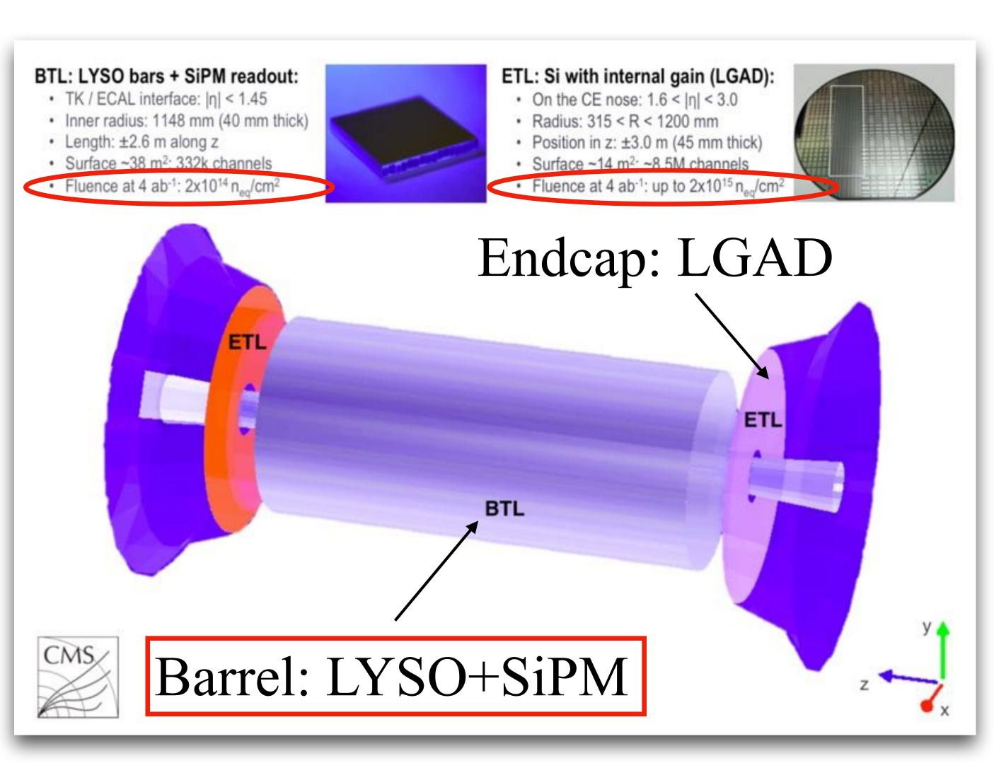
Different levels of radiation fluence in barrel and endcaps
