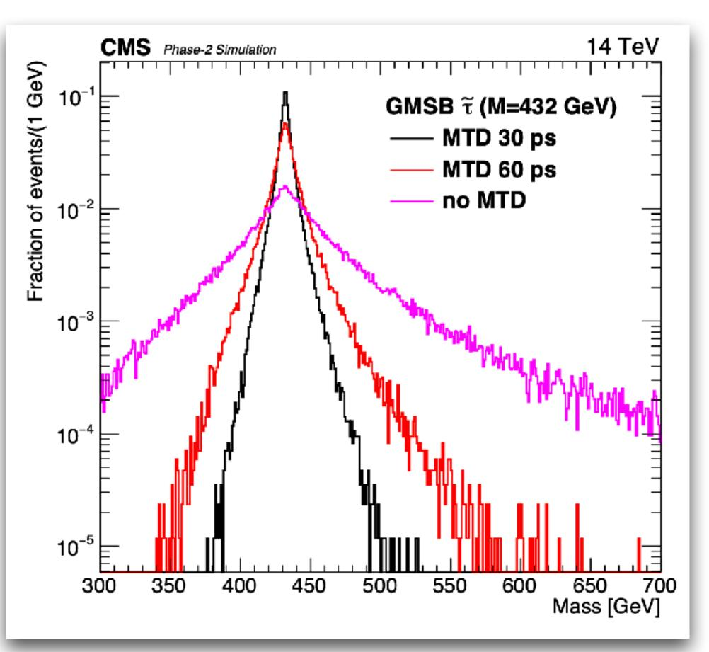
MTD impacts the resolution of the reconstructed HSCP mass significantly GMSB stau here has a very long lifetime crossing the full detector
