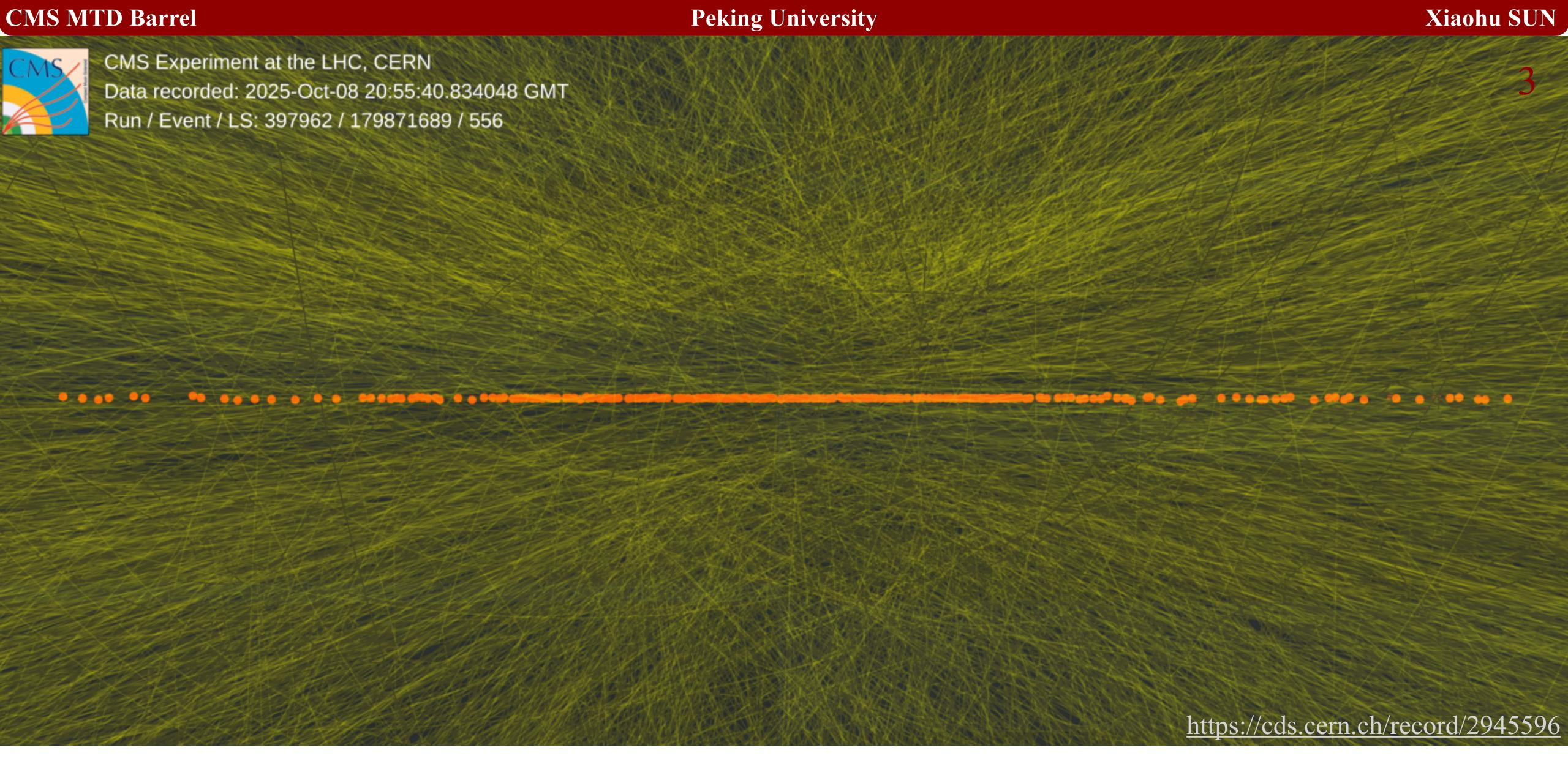
This is from a high-pileup run in 2025 with 206 vertices amongst the 9381 reconstructed tracks at one collision
