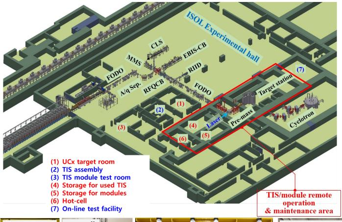
Proton cyclotron of 70 MeV and 50 kW (tested)
