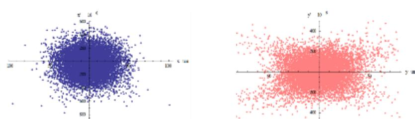
Beam distribution @ FF ( $\sim 20\mu\text{m}$ )
