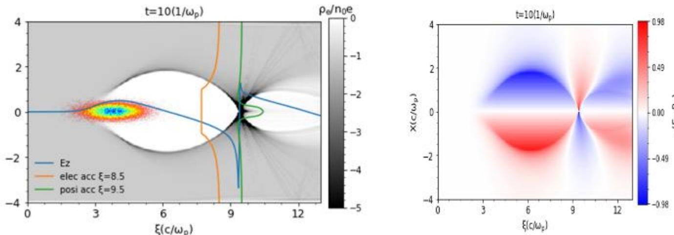
So, the blowout wakefield in uniform plasmas is quite fit for e- acceleration, while unfit for e+ acceleration
