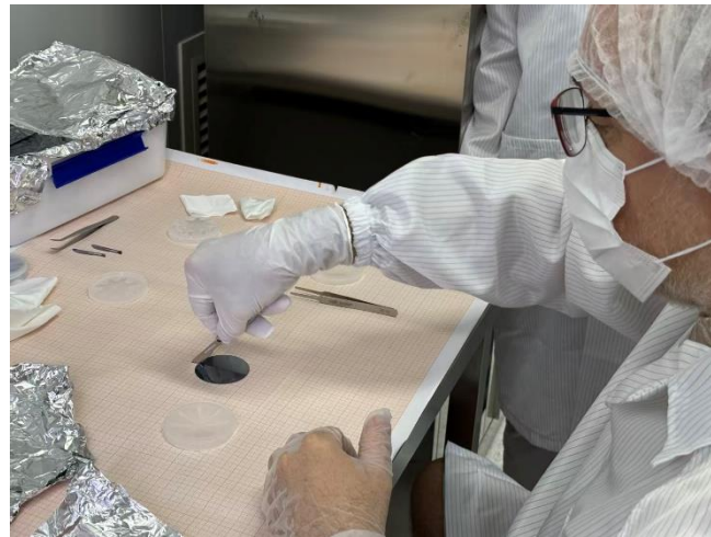
Superlattice GaAs wafer cut in Acken
