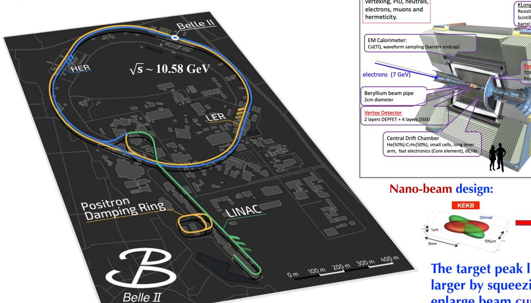
A multipurpose HEP The Belle II Detector spectrometer with vertexing, PID, neutrals, KLong and muon detector: Resistive Plate Chambers (barrel outer layers) Scintillator + WLSF + SiPM's (end-caps, inner 2 Particle Identification TOP detector system (barrel) Prox. focusing Aerogel RICH (fwd) positrons (4 GeV)
