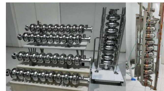
TESLA-Type Large-Grain 9-Cell Superconducting Cavity
