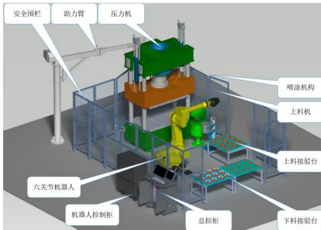
3D Layout of Stamping and Forming Automation Unit
