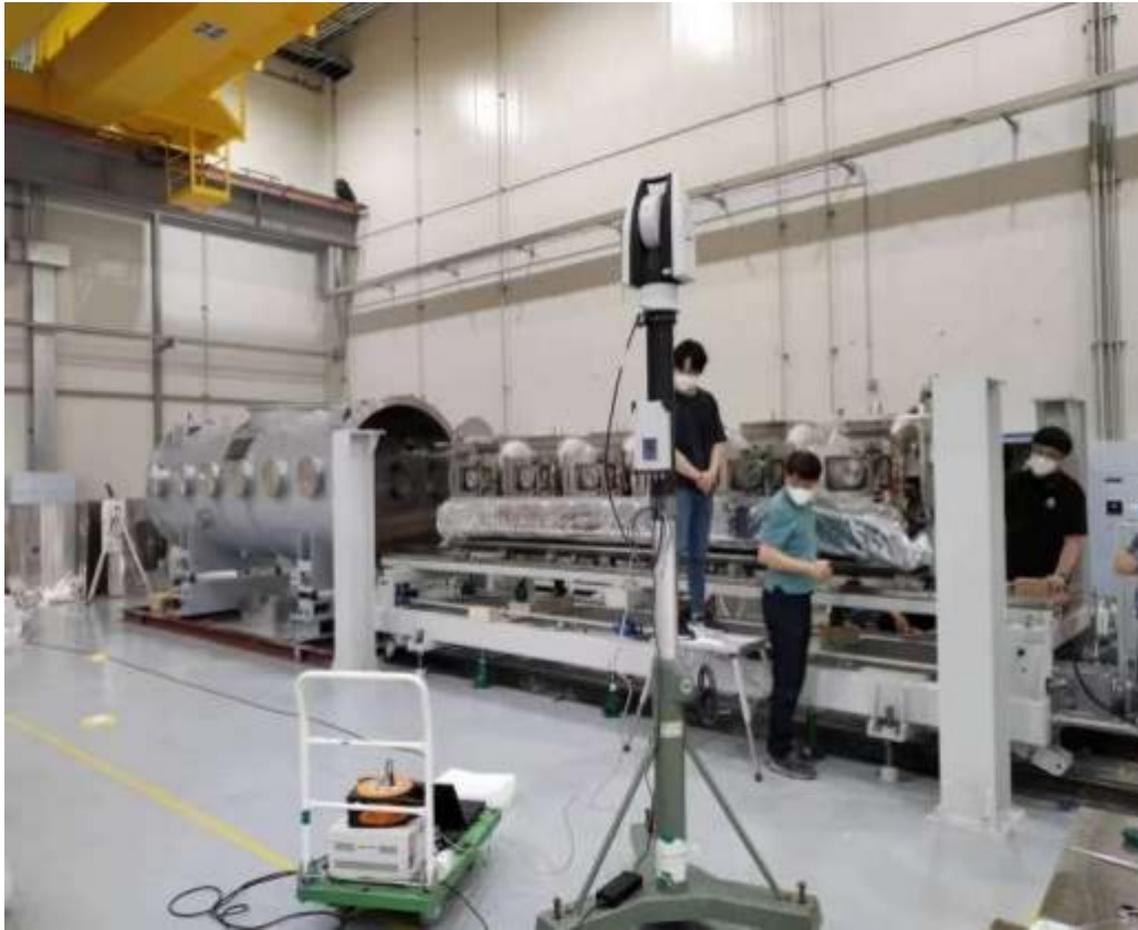
Cavity string alignment
