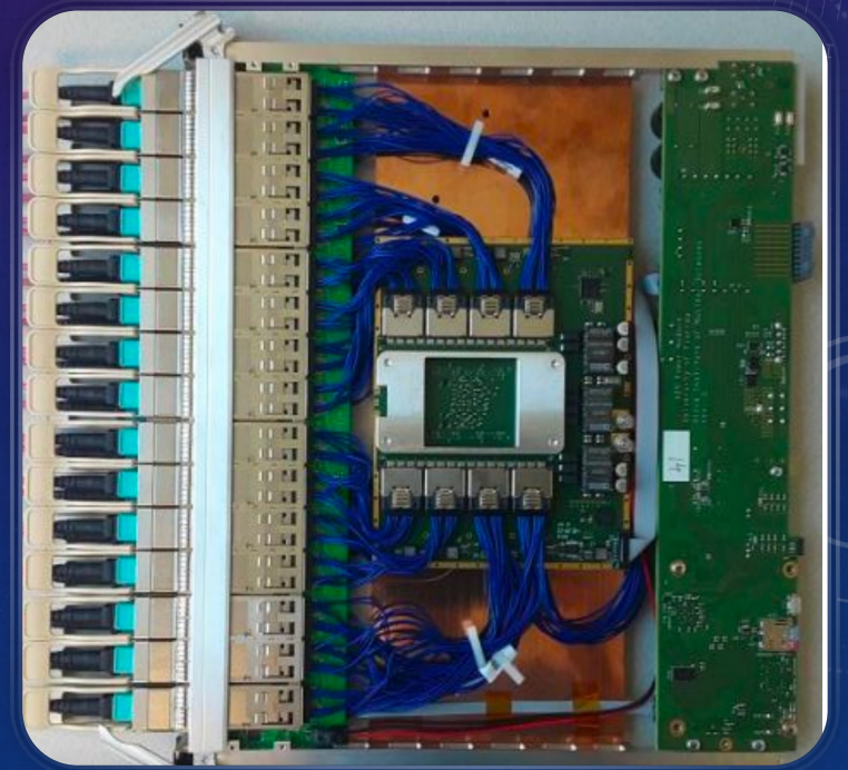
X2O modules attached to heatsink
