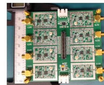
An 8-channel prototype frontend board made with COTS, read out using an oscilloscope
