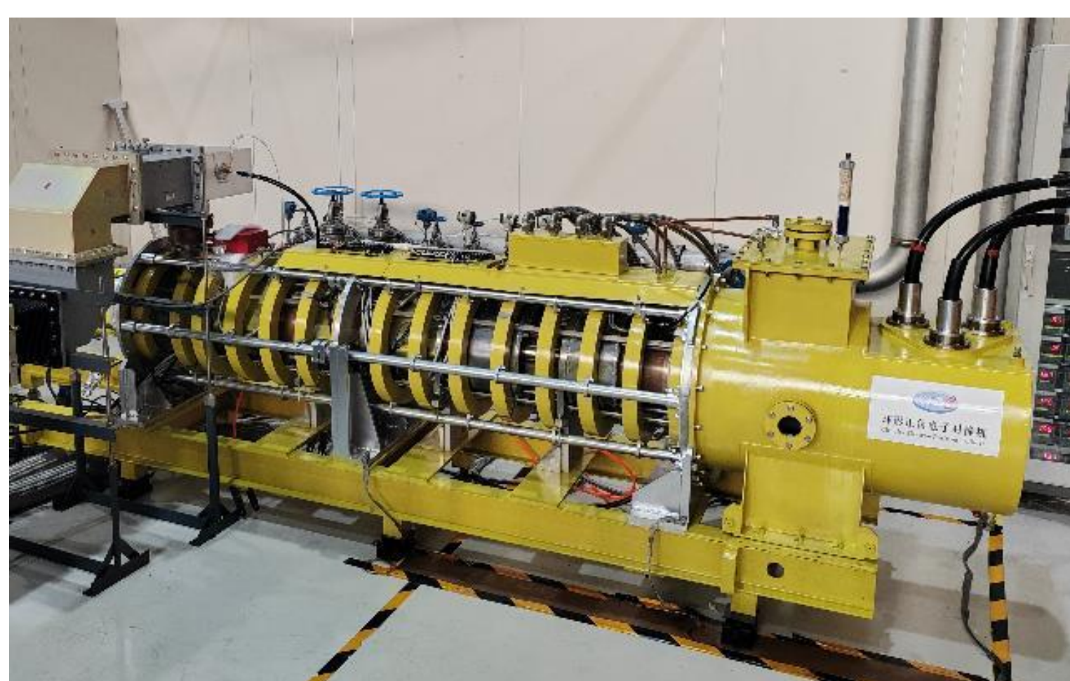
Fig.2. CEPC P-band high-efficiency klystron
