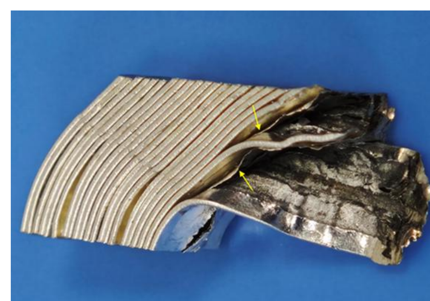
Figure 6. Photograph of the cross-section of the IBS-NI coil after heat treatment.
