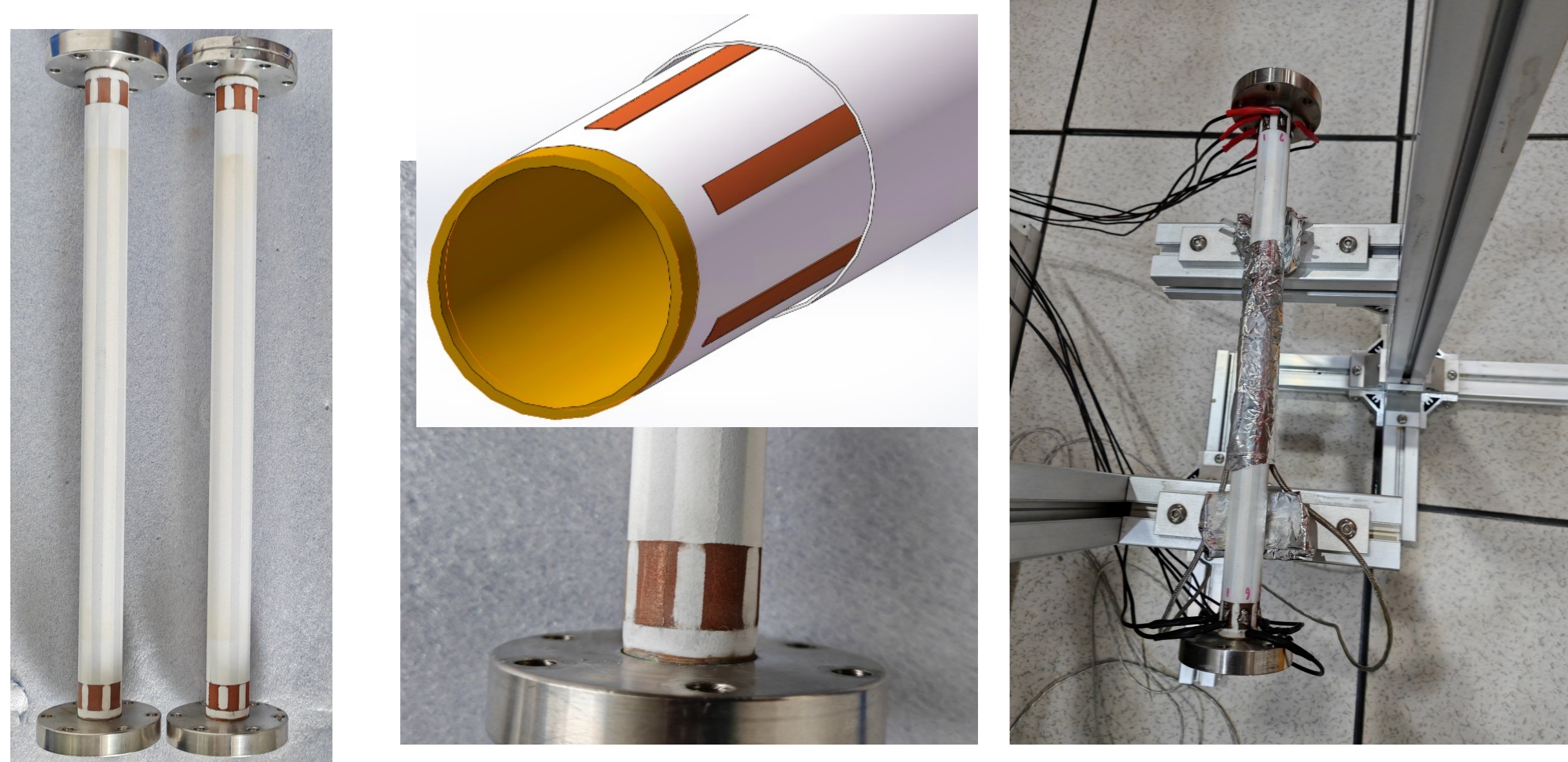
Multilayer thermal coating outside of vacuum chamber
