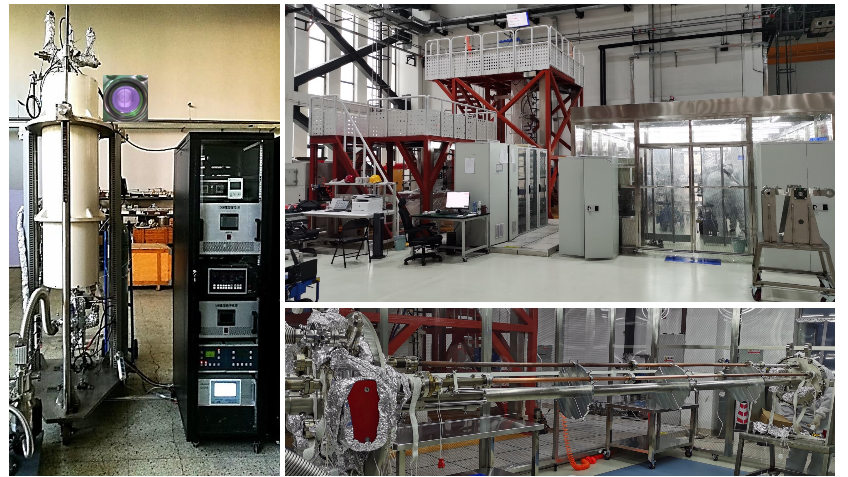
Prototype of NEG coating facility Massive production facilities of NEG coating
