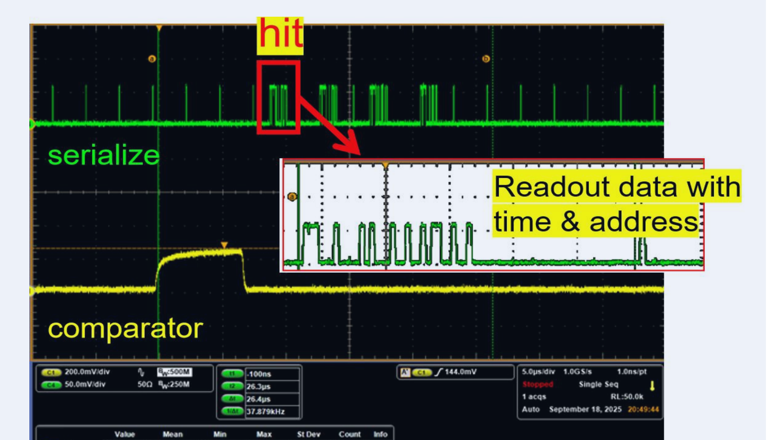
Fig. Response of full readout chain with laser test: Sensing diode → in-pixel (CSA/comparator/TDC) → EoC (digital peripheral) → data link → DAQ (refer to Boxin Wang's Poster)
