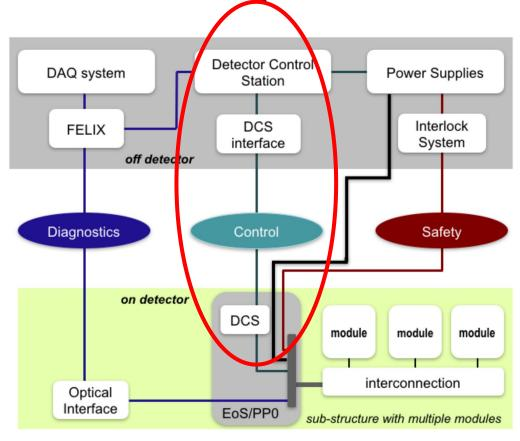
Figure 11.3: Overview on the ITk Pixel Detector Control System.
