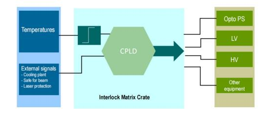
Figure 12.2: Schematic view of the Interlock Matrix Crate.
