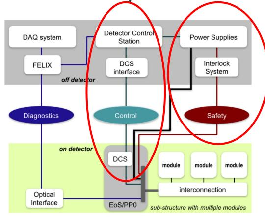
Figure 11.3: Overview on the ITk Pixel Detector Control System.
