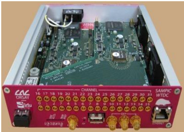
SAMPIC: TDC ASIC allowing to reach 3 ps time resolution
