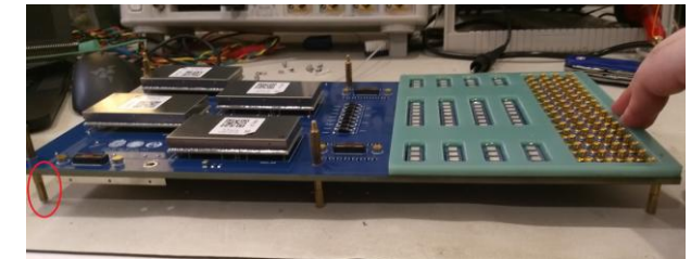
HV splitter: supply high voltage and split signal (Chile, Russian)
