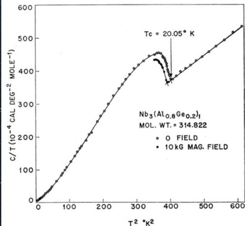
Fig. 1. Specific heat of Nb<sub>3</sub>Al<sub>x</sub>Ge<sub>1-x</sub> without magnetic field and with 10 kG.
