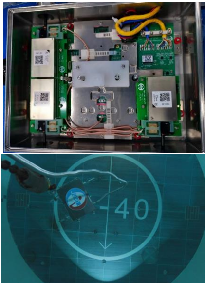
3 20-inch PMTs connected to one underwater box
