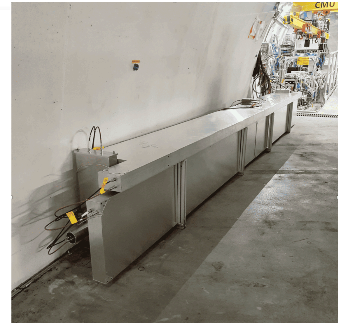
FORMOSA demonstrator 2x2x4 arrays of 5x5x80 cm 3 scintillator bars
