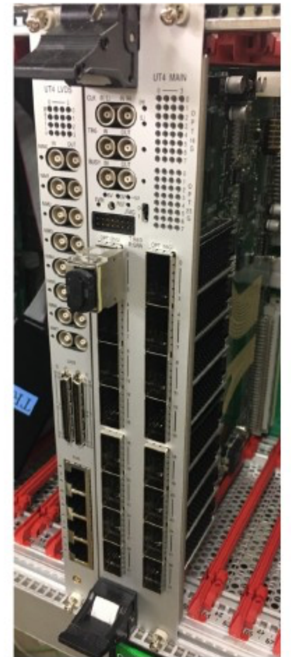
Xilinx UltraScale XCVU080, XCVU160 25 Gbps with 64B/66B
