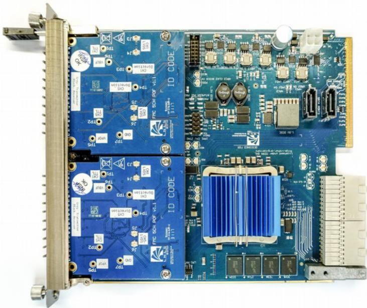
Figure 1: AFC board with two FMC 5 POF mounted.
