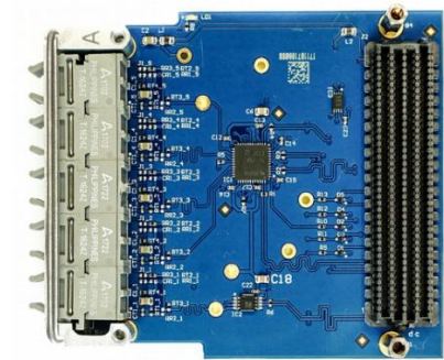
Figure 2: FMC 5 POF, a FMC board with 5 plastic optical fiber outputs.
