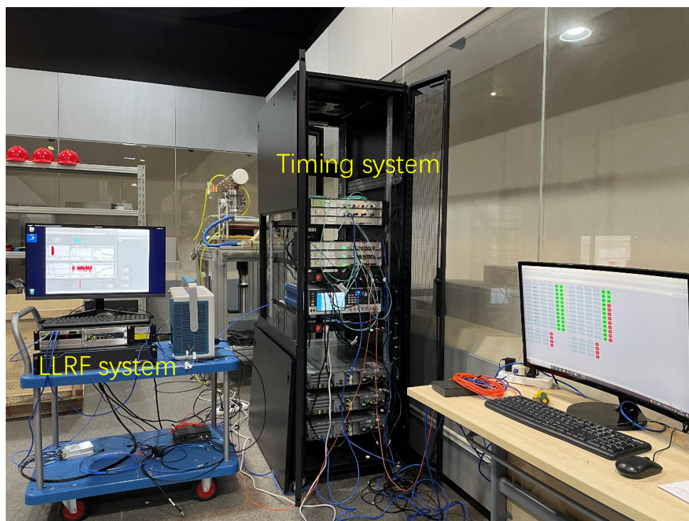
Integration test of LLRF & Timing system
