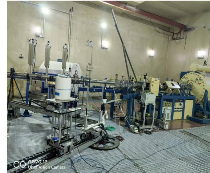
Calibration test of neutron dosimeter
