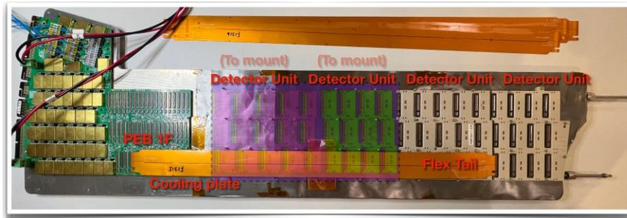
HV, LV, Cooling plate prototype
