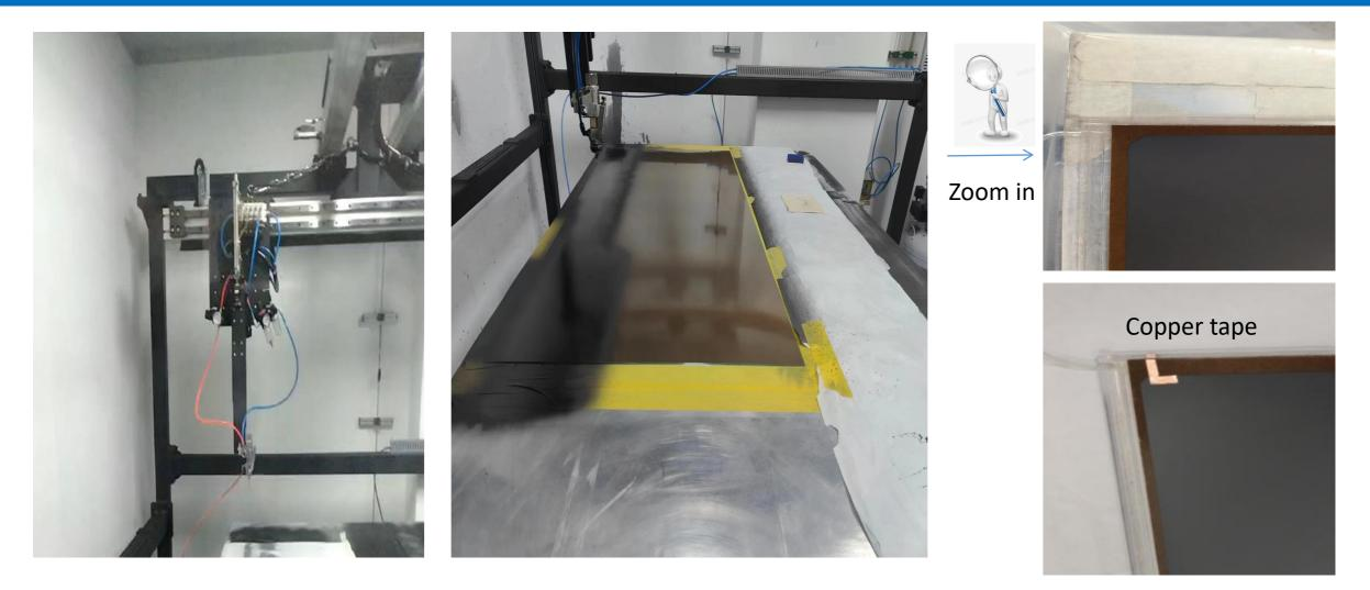
Graphite spraying system: A spray gun held on a 2-D gantry
