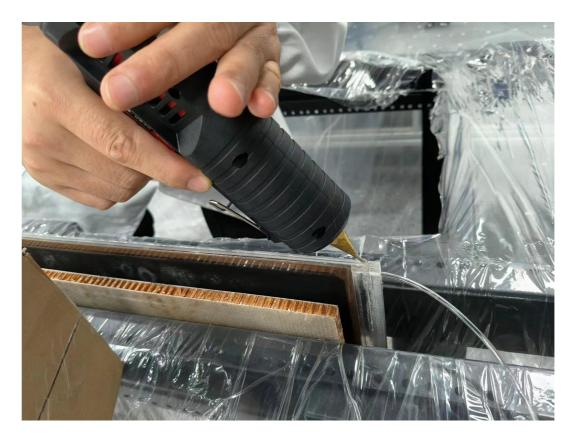
Filling and sealing the edges of the gas gap with hot-melt glue
