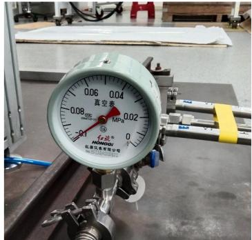
Keep at least 6 hours for the epoxy curing within the vacuum bag.
