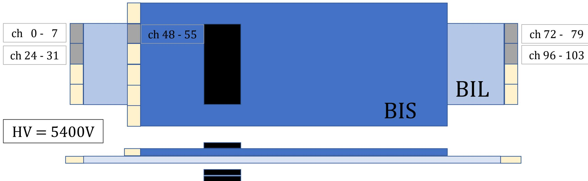
**Trigger System:** three scintillators operate in coincidence to generate the external trigger signal.
