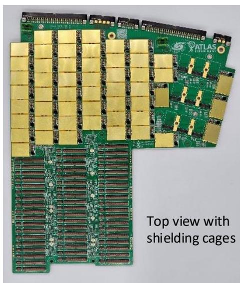
Top view with shielding cages
