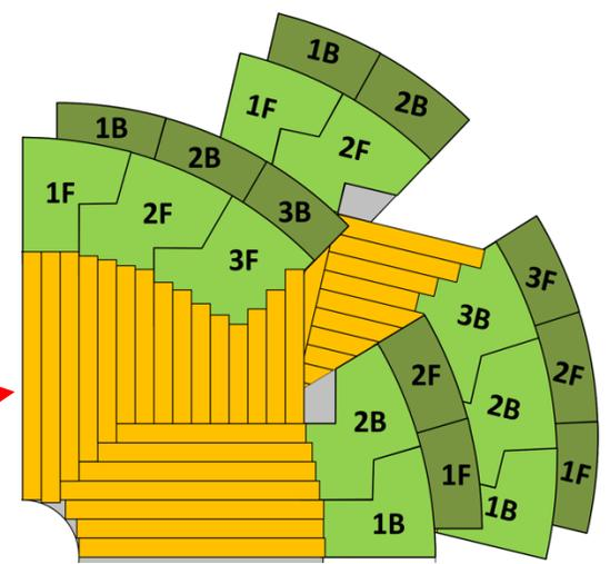
One quadrant of the two instrumented disks. The PEBs (in green) are attached to the readout rows
