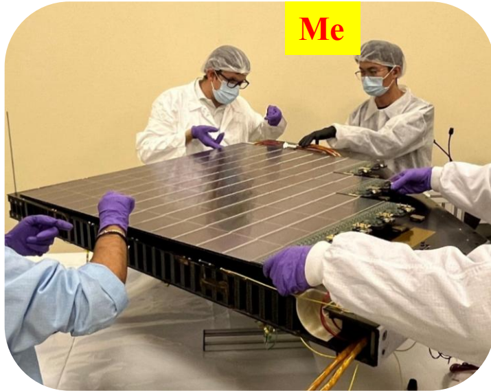
Ladder reception and \frac{1}{4} Layer assembly in Italy
