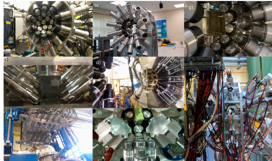
Fig. 14. (Colour online) Different setups in which the FATIMA detectors described in this paper have been mounted and used in experiments or tests. (a) At Argonne National Laboratory with half of the Gammasphere array. 25 detectors mounted in a hemisphere. (b) At the University of Surrey, some detectors are mounted on the DESPEC FATIMA frame in its core configuration with space for 36 detectors on three rings. (c) At GANIL at the LISE station together with HPGe Clover detectors. (d) At IPN Orsay during the v-Ball campaign 2017/2018. (e) At IPN Orsay for the Stella experiment. 36 detectors in a semi-cylindrical configuration. A manual lift system with counter-weights is used to allow access to the target chamber. (f) At RIKEN during the EURICA campaign. The detectors have been placed in free spaces in the array in clusters of six. (g) and (h) At GSI in the S4 cave in the configuration designed for use in the DESPEC station for FAIR (AIDA snout and rack to the left, beam from left to right).
