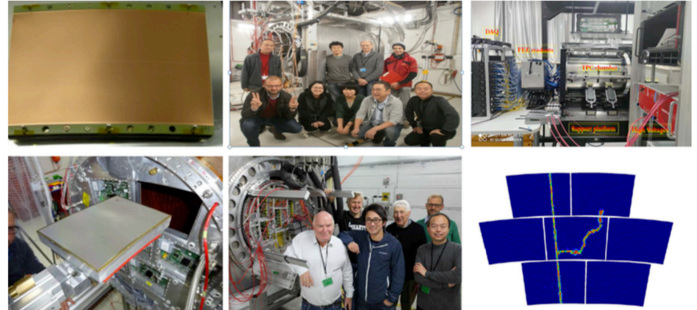
Figure 6.20: Beam tests of TPC prototype at DESY in LCTPC international collaboration, the performance of the prototype was evaluated in a beam test using 5 GeV electrons from several R&D groups in the collaboration.
