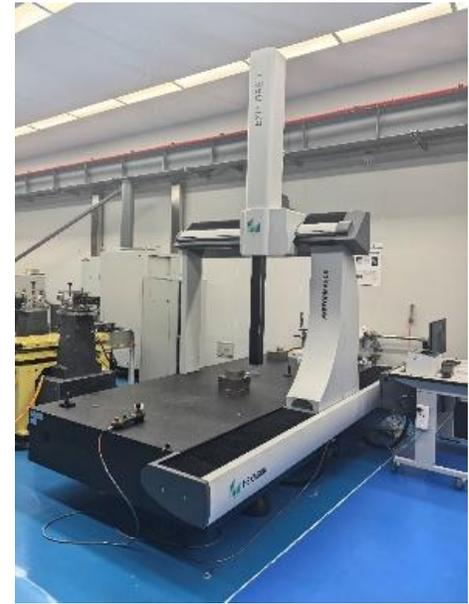
Hexagon bridge-type coordinate measuring machine (CMM)
