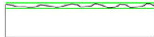
**Continuously** traversing a defined distance along the surface profile
