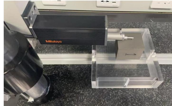
Probe-type: Surface roughness meter
