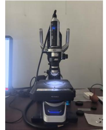
Optical-type: Ultra deep field 3D microscope
