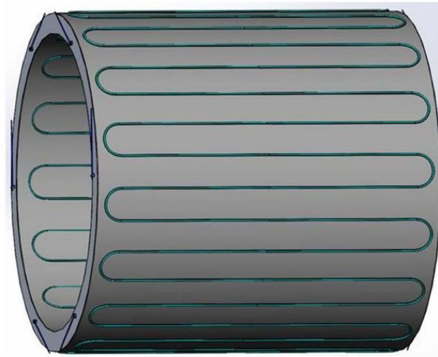
Figure 10.41: Structure of the thermal shield. The cooling is achieved by forced flow method using 40 K cold helium gas.
