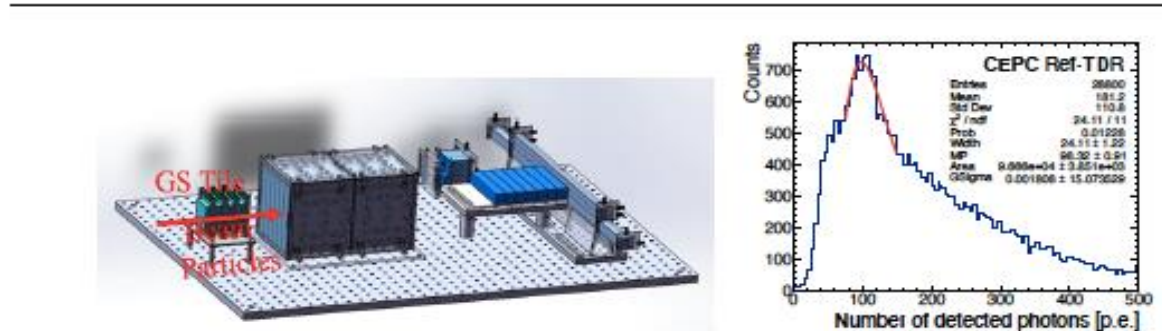
Figure 8.8: DESY electron beam test of the GFO glass tiles in 2023. Left figure shows the experimental setup, right figure shows the measured p.e. distribution.
