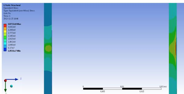
Figure 6: Stress distribution after 20 pulses in the two energy degraders of FC3 at 50 MeV (fast mode).
