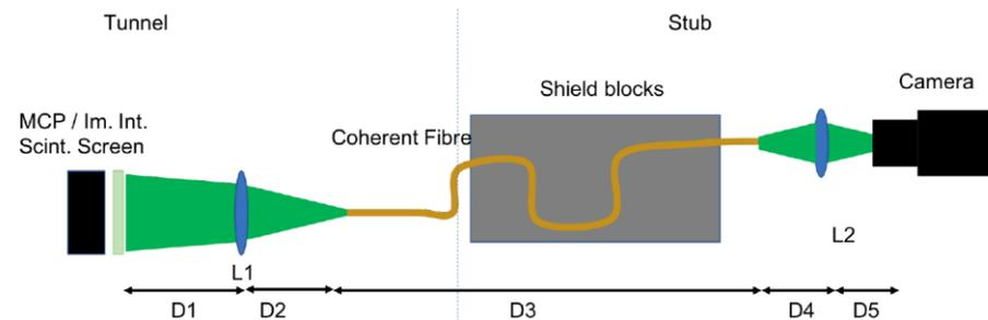
The fiber-based imaging layout
