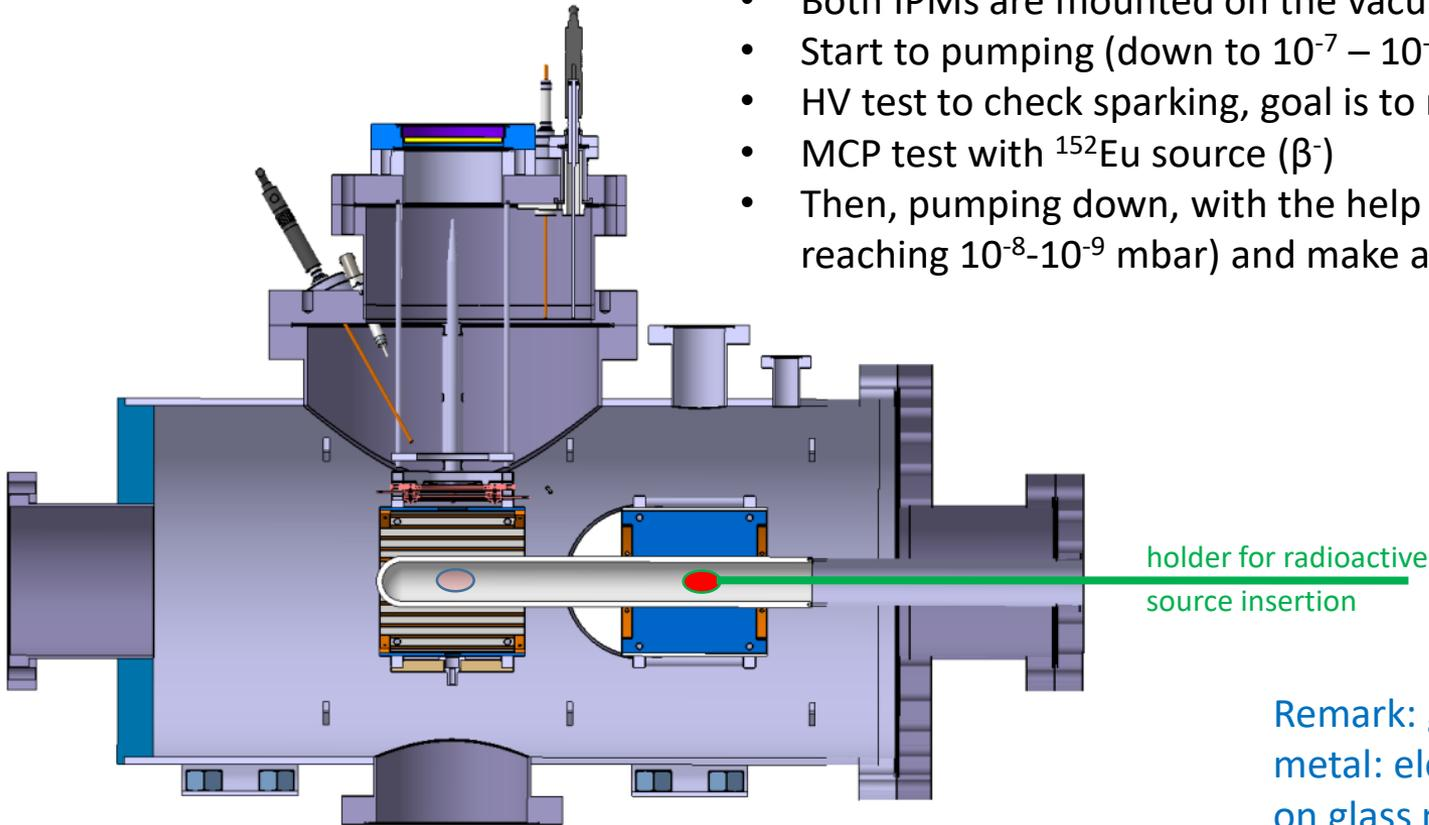
Remark: glass finger brazed on metal: electric charge loading on glass may induce sparks...
