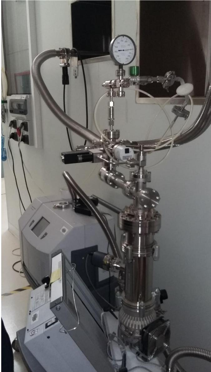
Slow pumping system and slow N<sub>2</sub> filling up to atmospheric pressure developed by DACM staff member for compliance with free particle requirement.
