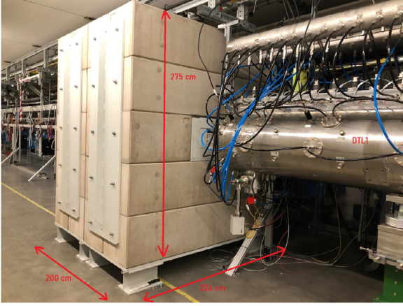
Fig. 5. The DTL1 FC shielding installed in the ESS accelerator tunnel.
