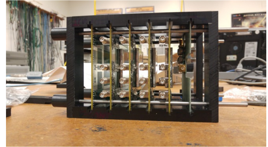
Stack of LGAD planes and the trigger plane
