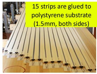
Three segments (15 strips each) have fallen down inside the detector due to the weak fixation. Two were repaired.
